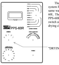
The measurements with the system PPS -60R can be done in the same way as with the system PPS-60L. The only difference is that in PPS-60R there is an additional switch allowing to choose one of 5 drying chambers.
