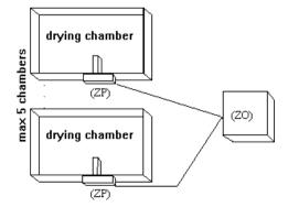
Only the transducers (ZP) are located on the wall outside of the drying chamber and the receiver (ZO) can be located up to 100m from the chambers. Five transducers (ZP) can be connected to one receiver (ZO).
